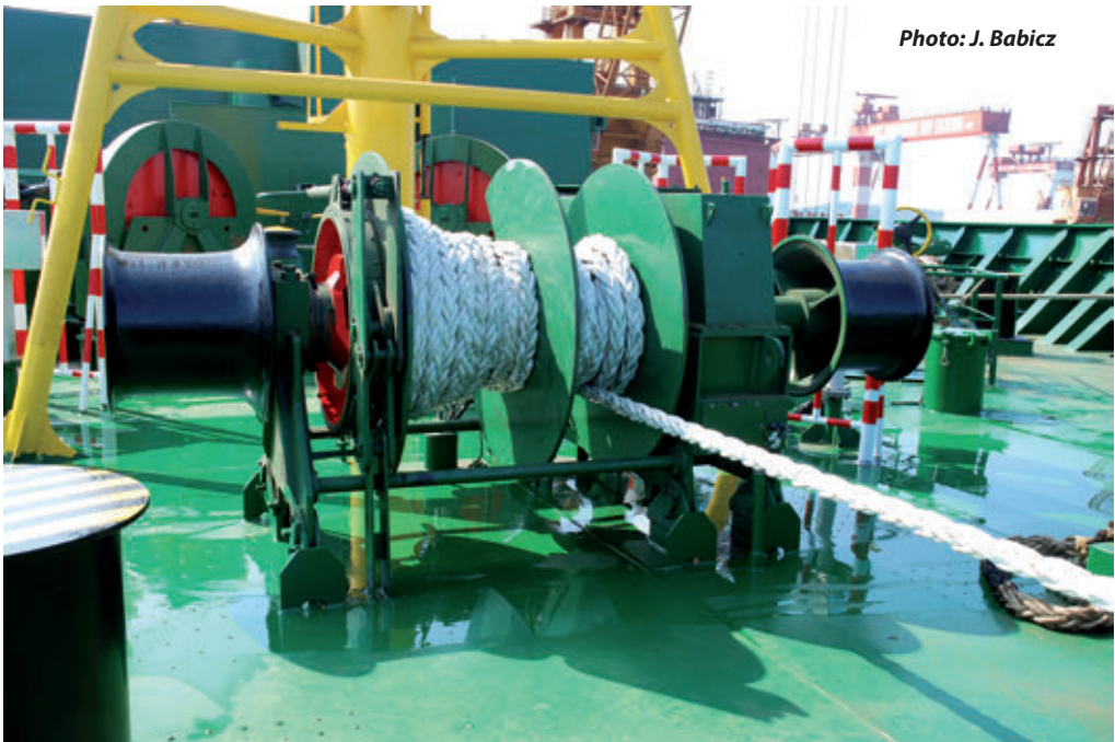
Electrically driven mooring winches with two split drums
