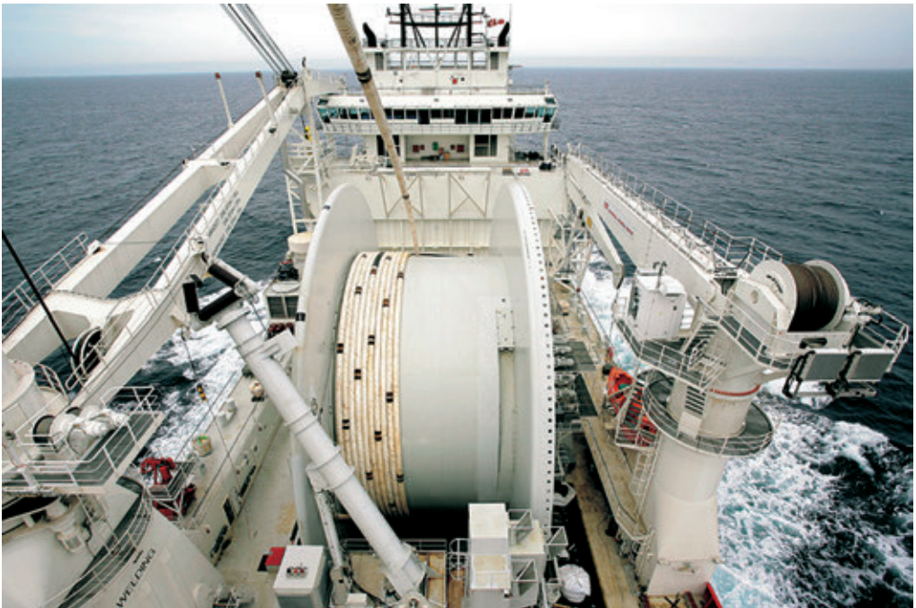
The 28-meter diameter reel weighs more than 900t, making it the largest reel which has ever been made. The quantity of steel which can be transported on the reel – 3500t – is also a new record
