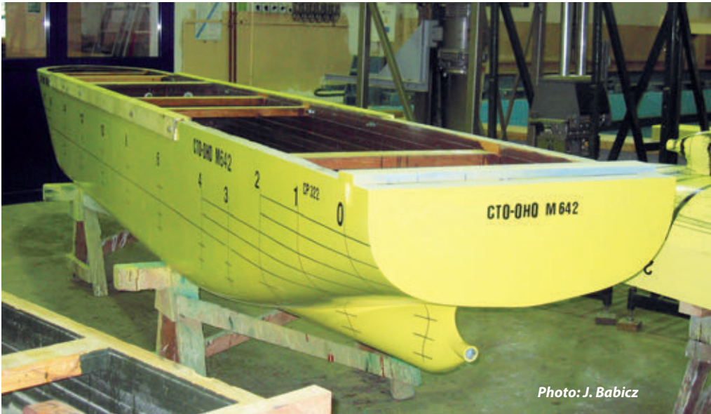
The model of the MPV OSTSEE in the Gdańsk Ship Model Basin CTO S.A. Hull shape designed by BOG-Projekt
