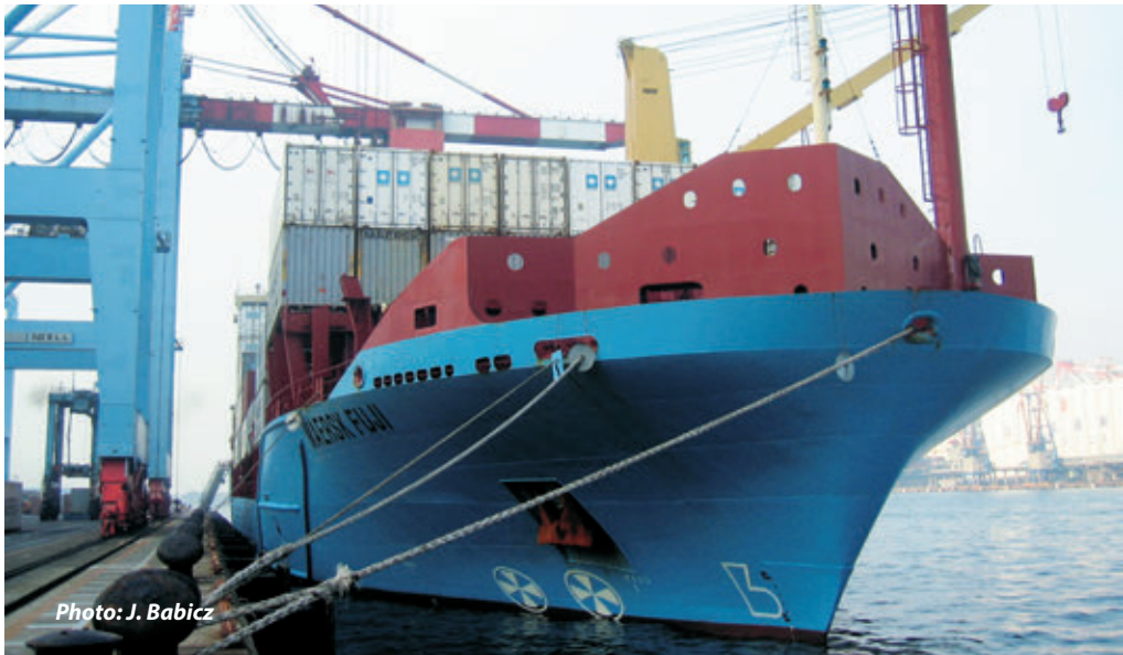
New type of the breakwater applied by Jan Babicz. Such breakwater protects not only cargo but windlasses and mooring winches as well
