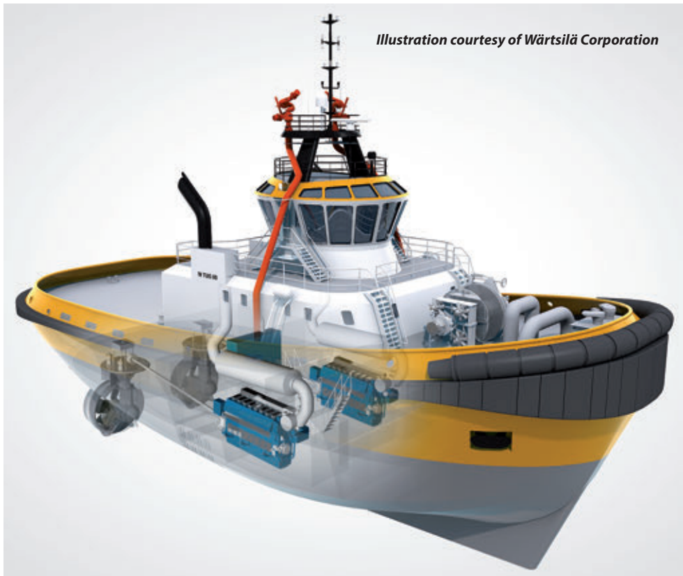
Escort tug W TUG 80 designed by Wärtsilä bollard pull 80 tonnes, speed abt. 14 knots, L OA 35.40m
