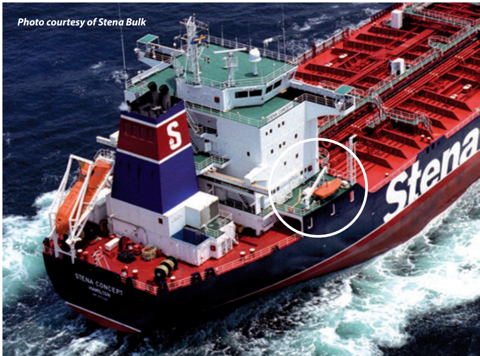
Right arrangement of rescue boat, far away from the propeller, high enough to be protected from damage by heavy seas
