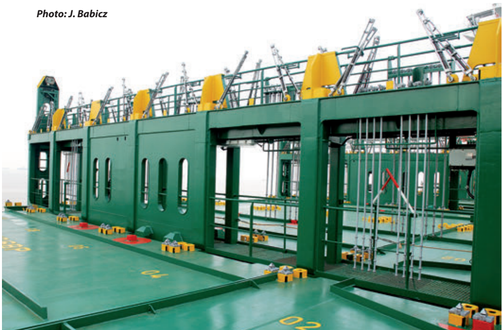
Lashing bridge on CV 5300 TEU
