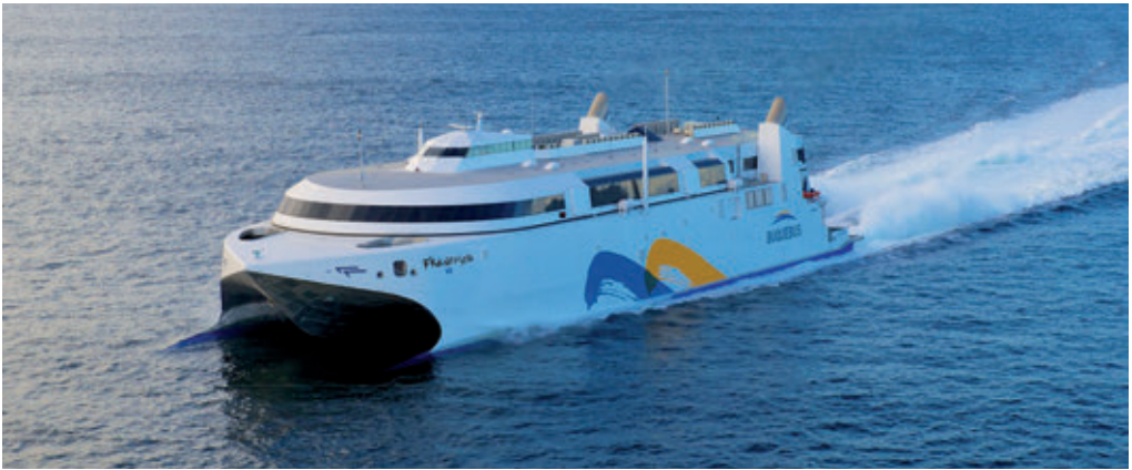
FRANCISO is the first dual fuelled fast ferry to operate with LNG as the primary fuel
