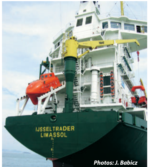
Free-fall lifeboat and simple launching ramp. Recovery by a combined life-saving/provisions crane
