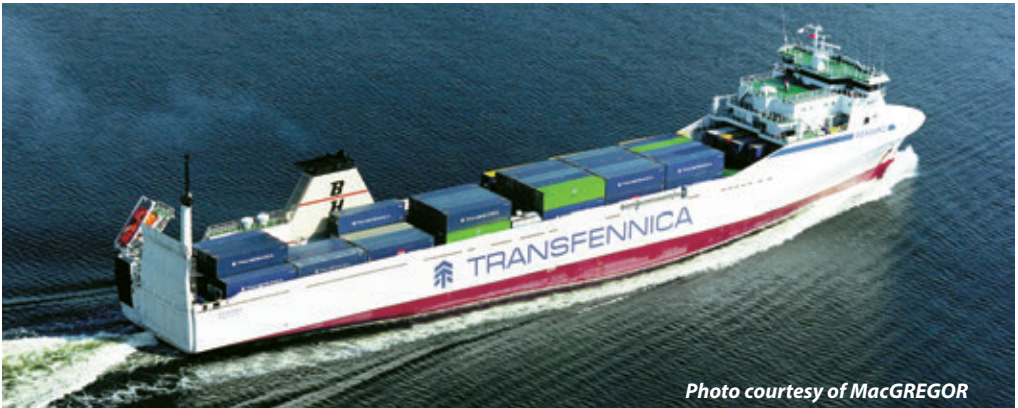
Wrong location of lifeboat far-away from accommodation
