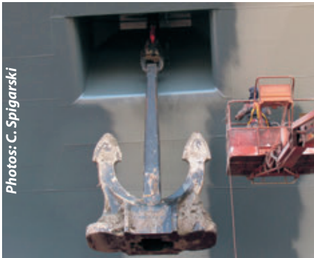
Spek anchor, note anchor pocket
